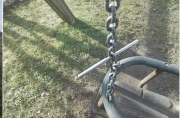
Finding: The chain openings are in excess of 8.6mm and do not meet the recommendations of BS EN 1176 Part 1
